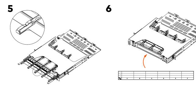
**Tip** At the front of the panel, place the cables in the hoops to ensure that they are properly routed to the left or right.
