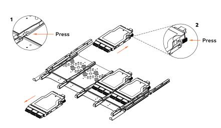
The fiber cassettes can be removed and installed from the front or back of the panel, depending on the space available.
