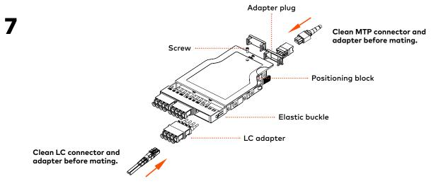
To ensure the optimal functioning of your structured network, please note the importance of cleaning the connectors before inserting them into the fiber cassette.
