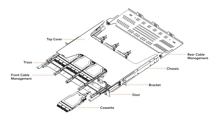
barpa's Fiber Optic UHD Panel is pre-configured for 12-fiber cassettes. For each U, there are 3 trays that hold 4 cassettes of 12 fibers each.
