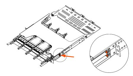
If necessary, each tray can be removed from the panel.
