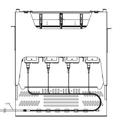
**Tip** On the back of the panel, route the cables to the left or right, as shown in the image, to ensure they are better positioned.
