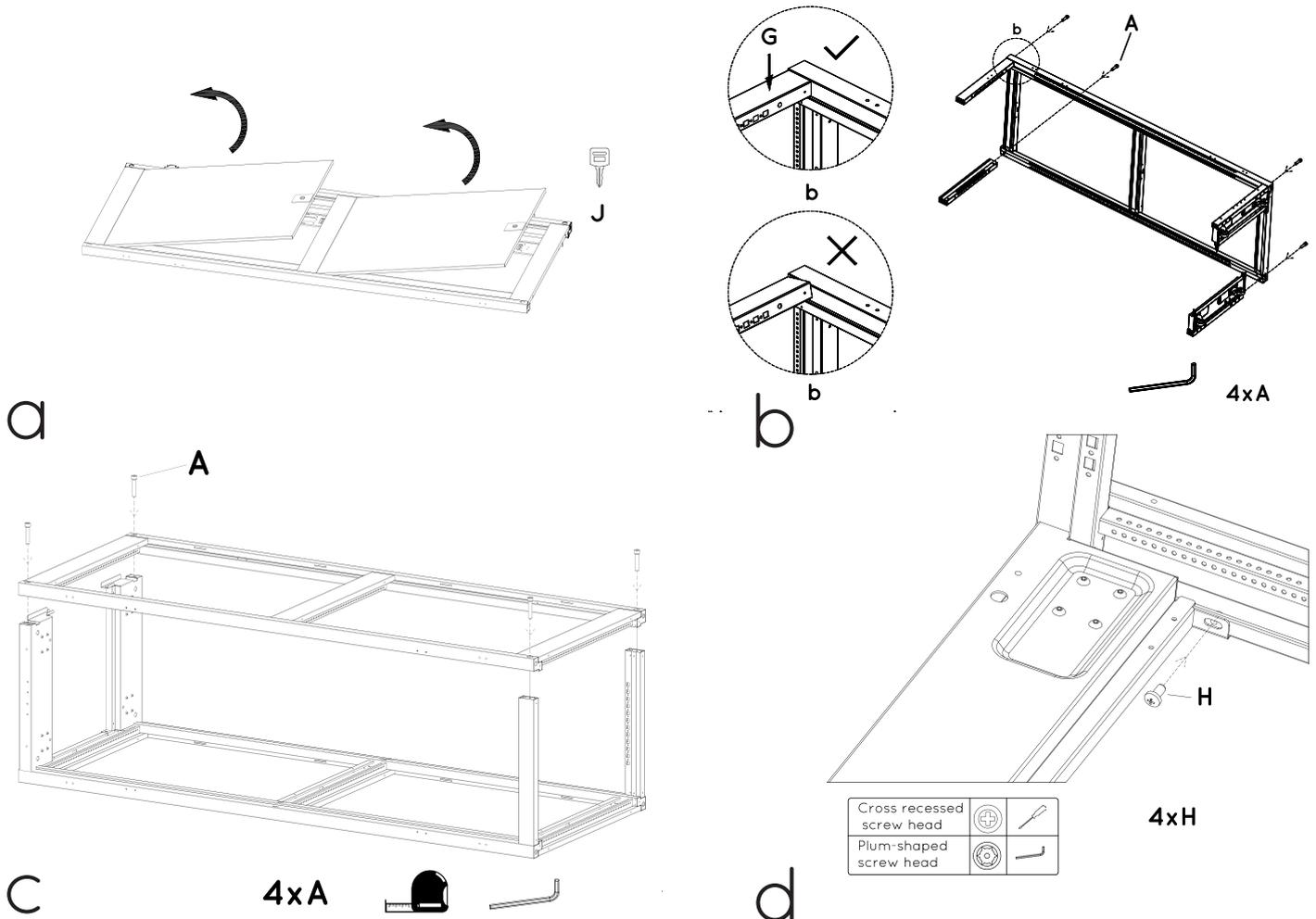
After assembling, if the diagonal framework is more than 4mm, it is required to loosen the bolts and then reassembled;
