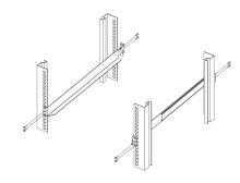
Screw the front flange to the rack first. Slide the bars with the rear flange towards the rack until the flanges make contact with the rack, then screw the rear flanges to the rack.
