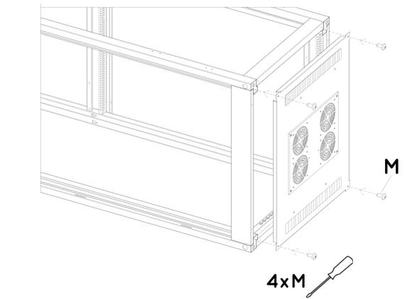
After assembling, if the diagonal framework is more than 4mm, it is required to loosen the bolts and then reassembled;
