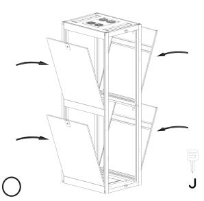
When assembling the side panels, it is necessary to lock the panels and remove the keys in case of falling down!
