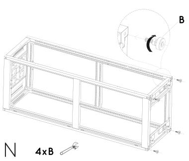
After assembling, the M12 feet should be under (shorter than) the castors in case of breaking when set up the cabinet!
