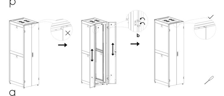
Doors can be adjusted by loosening hinge screws, moving the door and retighten.
